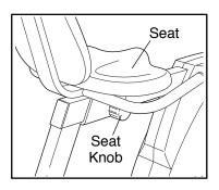
adjust the seat, make sure that your knees will not touch the handlebar or the console when you pedal. To adjust the seat, first turn the seat knob counterclockwise two or three turns to loosen it (if the seat knob is not loosened enough, it may scratch the frame). Next, pull the seat knob, slide the seat to the desired position, and then release the seat knob. Make sure to move the seat back and forth slightly until it locks in position. Then, turn the seat knob clockwise to tighten it.
